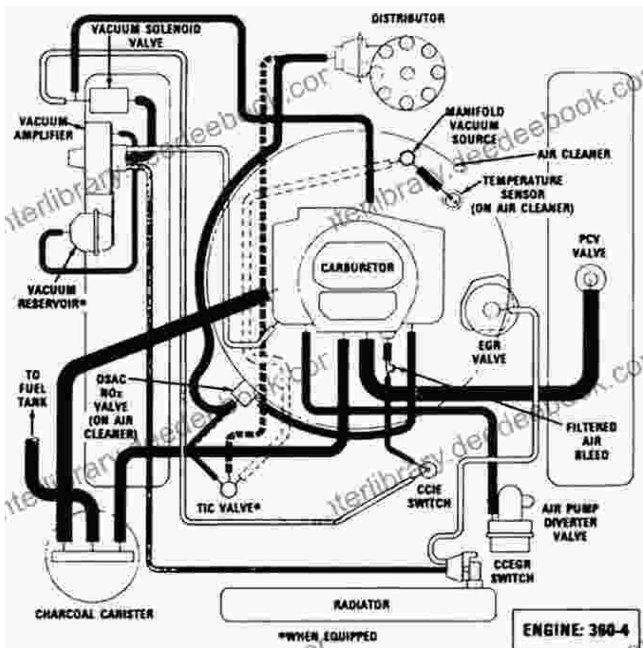
Focuses on the vacuum lines and components related to engine operation, such as the carburetor, distributor, and power brake booster.
